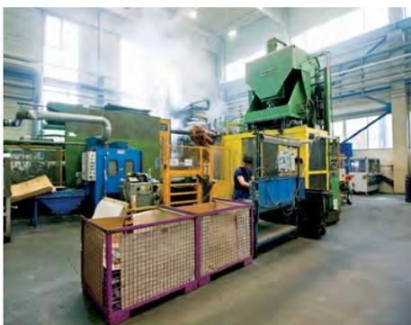
The semi-finished products of the foundry are stored in designated containers. As soon as a container is filled, it is equipped with a KANBAN card and transferred to the further processing department.
