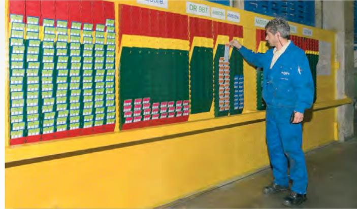
KANBAN boards fulfil several functions in the control loops. On one hand, they help with the sequence planning of the production orders activated by the cards, and on the other hand, they determine the priority level. For this reason, the compartments are painted in traffic-light colours. The cards that return first are sorted into the green compartments, then into the yellow and finally into the red ones.
